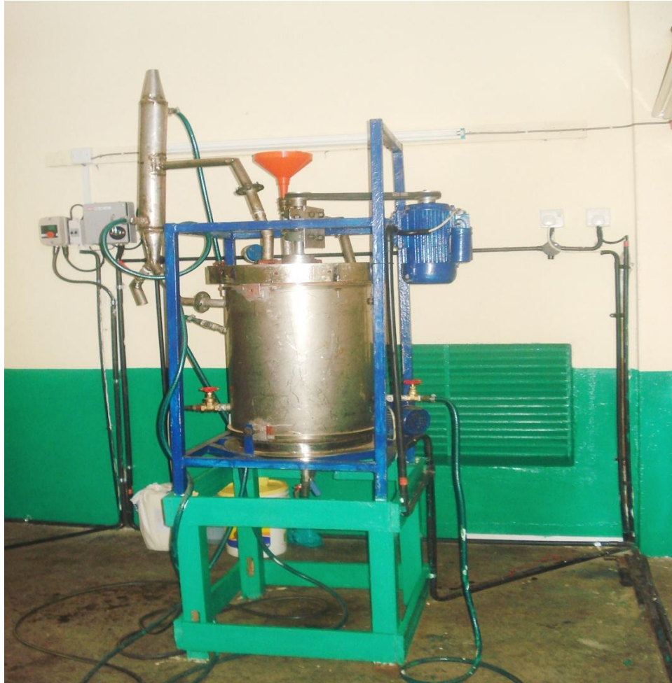
Plate 1. Transesterification reactor (Capacity 60 L /hr biodiesel)
