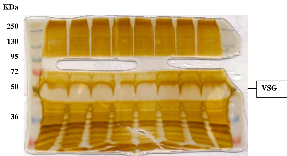
Figure 4 : Silver stained SDS-PAGE gel of complete trypanosomes lysate. All the lanes were loaded with 10 \mu\text{g} of protein. Also shown is an excision of the gel band between 72 and 95 KDa. The variant surface glycoprotein (VSG) of trypanosome was visualized at around 50KDa.
