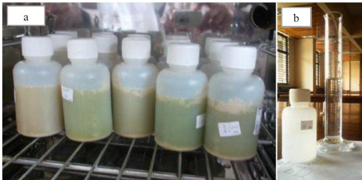
Figure 3. 4: Juice fermentation and, b) ethanol obtained after distillation
