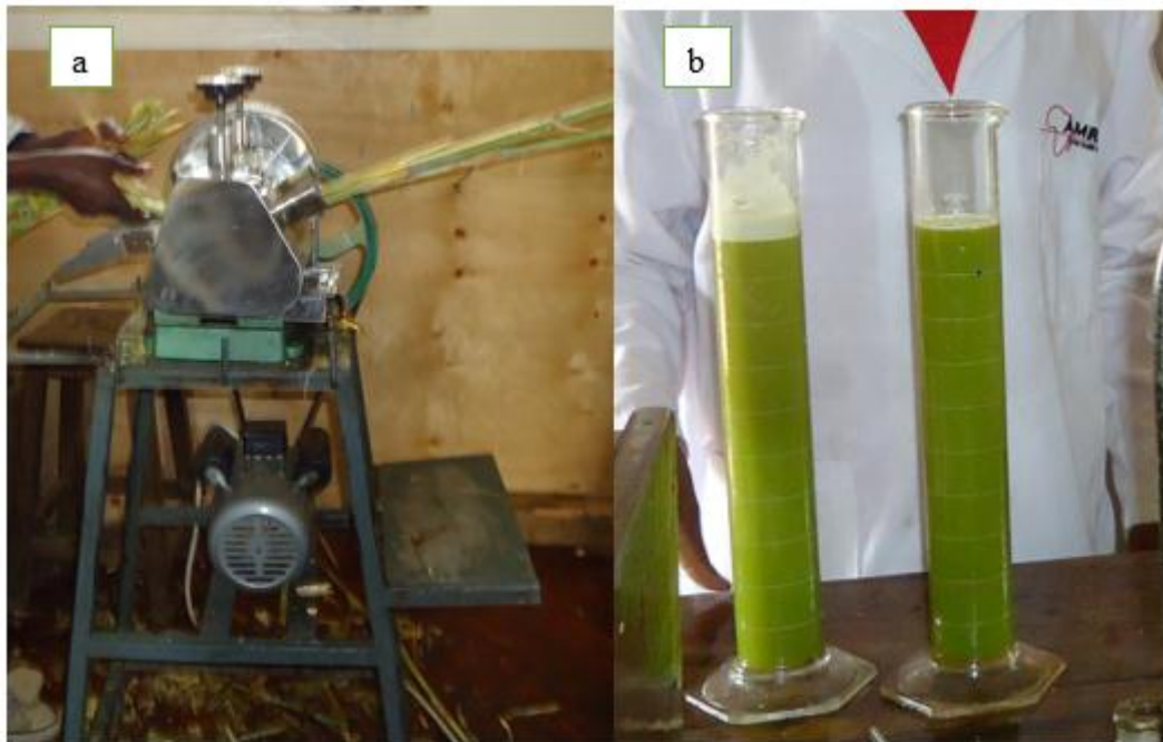
Figure 3.3: Juice extraction (a) and stem juice being measured (b)
