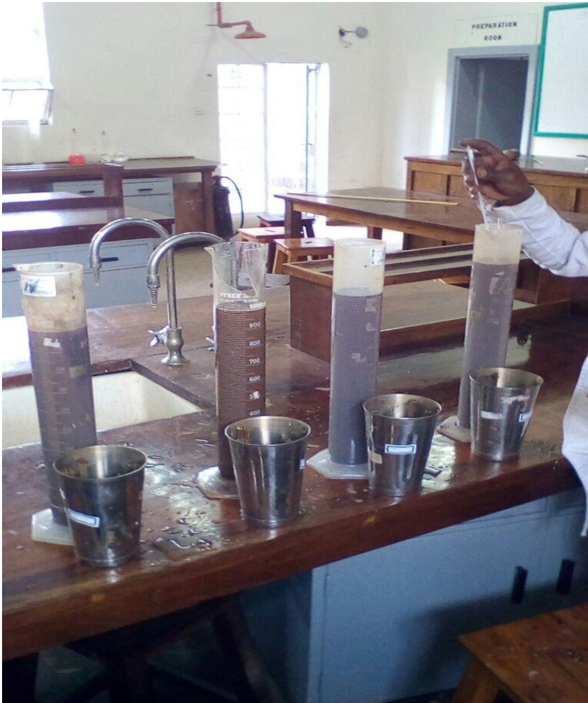
Appendix B. 1 : Soil texture determination
