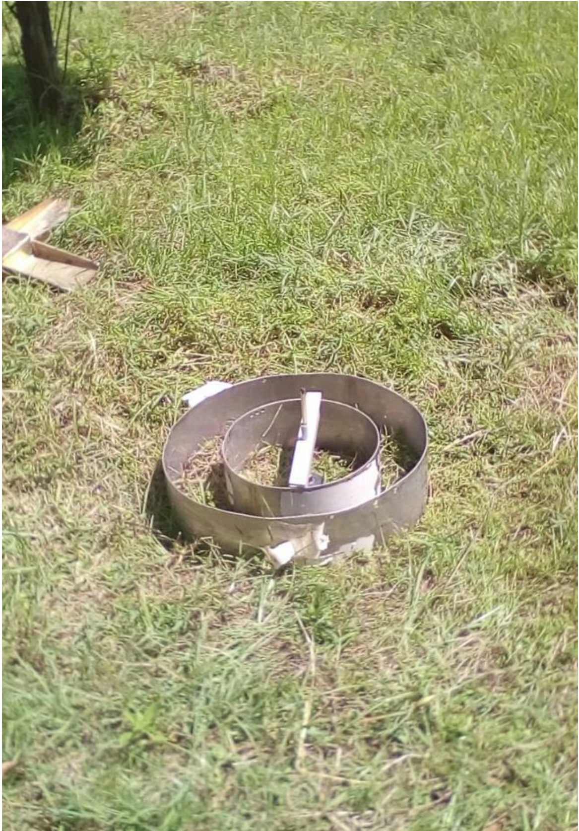
Appendix B. 4 : Infiltration test set-up
