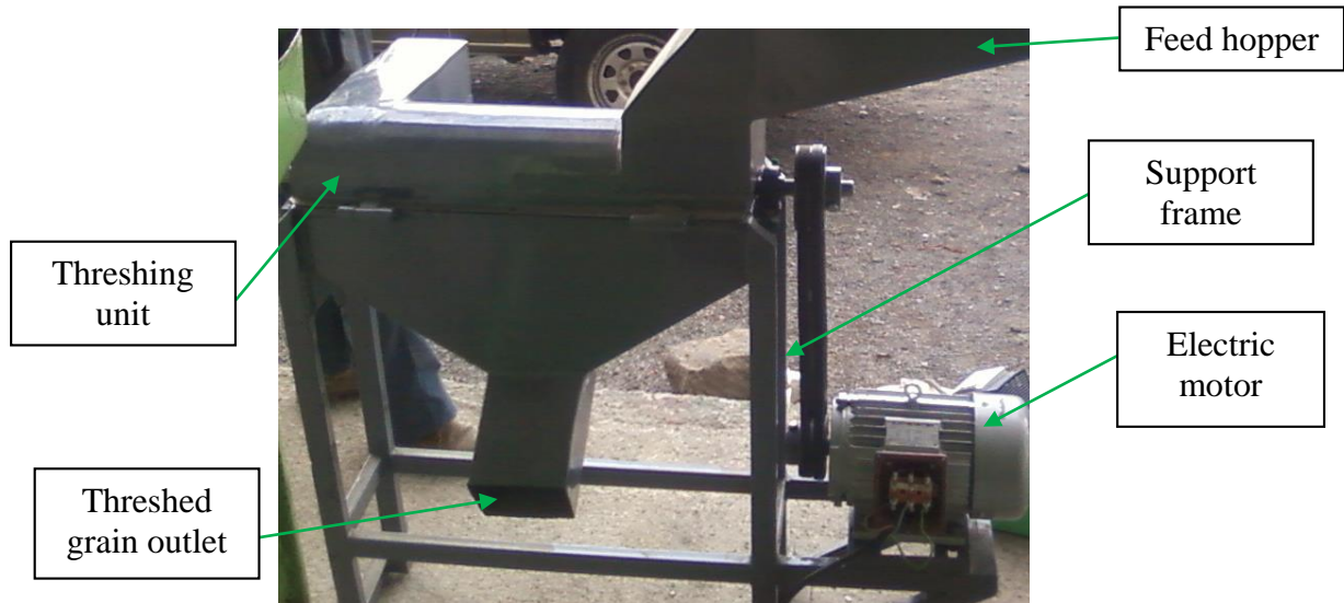
Plate 3. 2: The developed sorghum thresher
