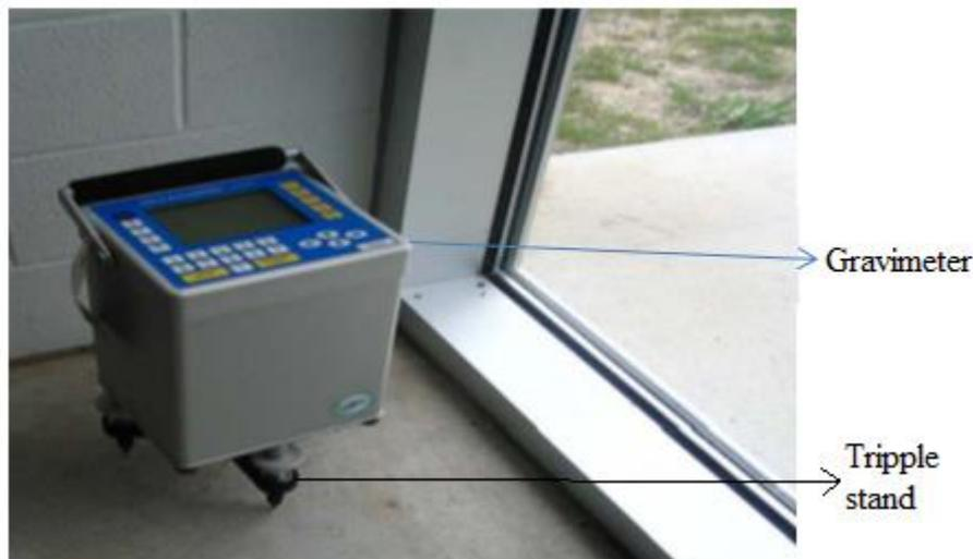
**Figure 2.1:** CG-5 Autograv gravimeter
