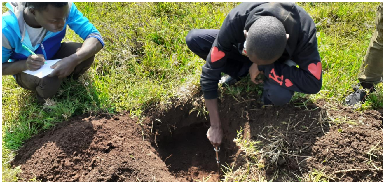
Plate 4.2: In situ determination of penetration resistance
