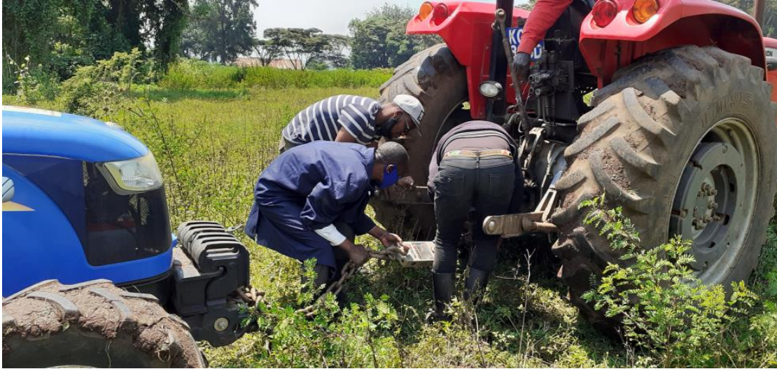
Plate 4.5: Connecting the dynamometer
