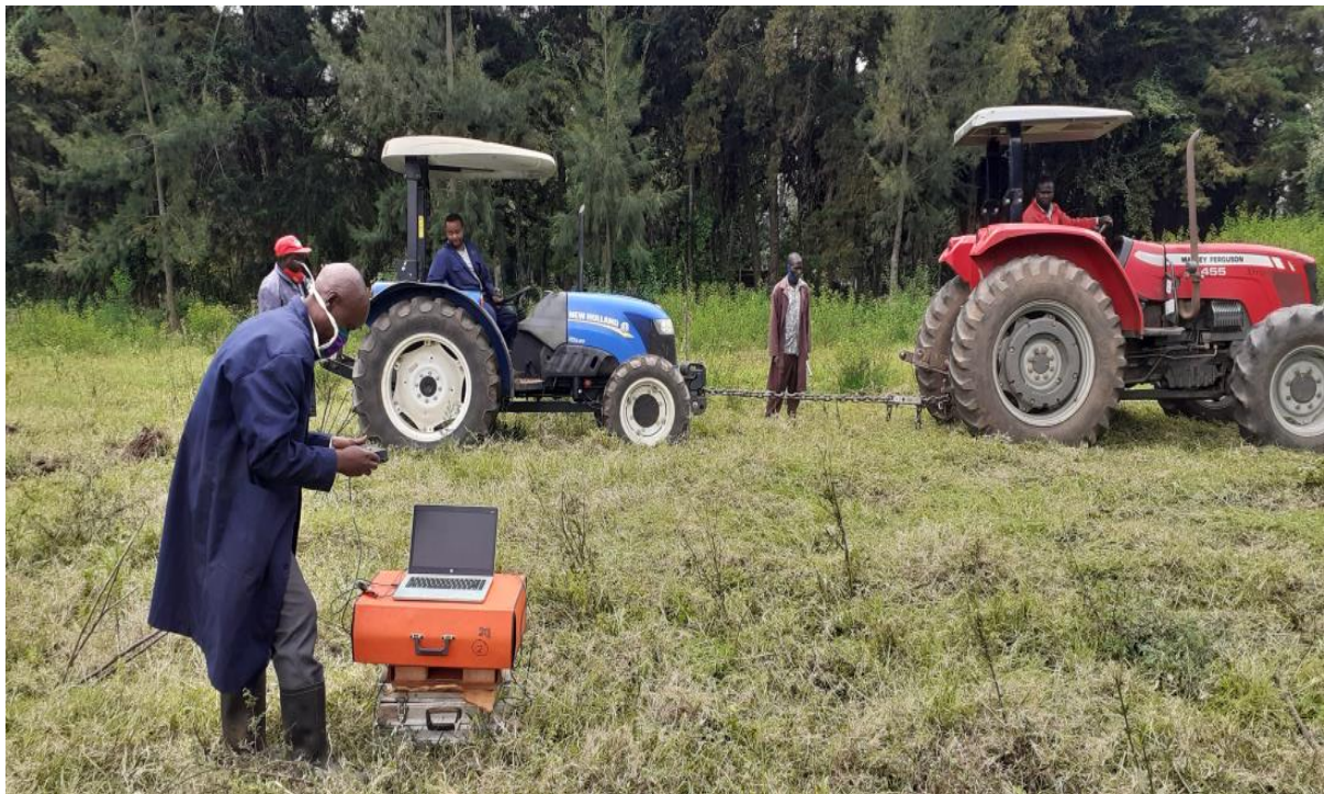
Plate 4.6: Subsoiling draft determination
