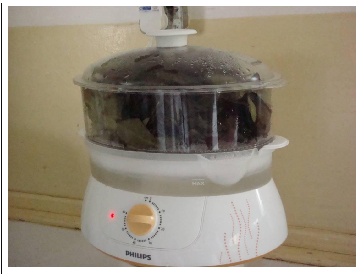
Figure 8: Modern steaming vessel used in green tea manufacture
