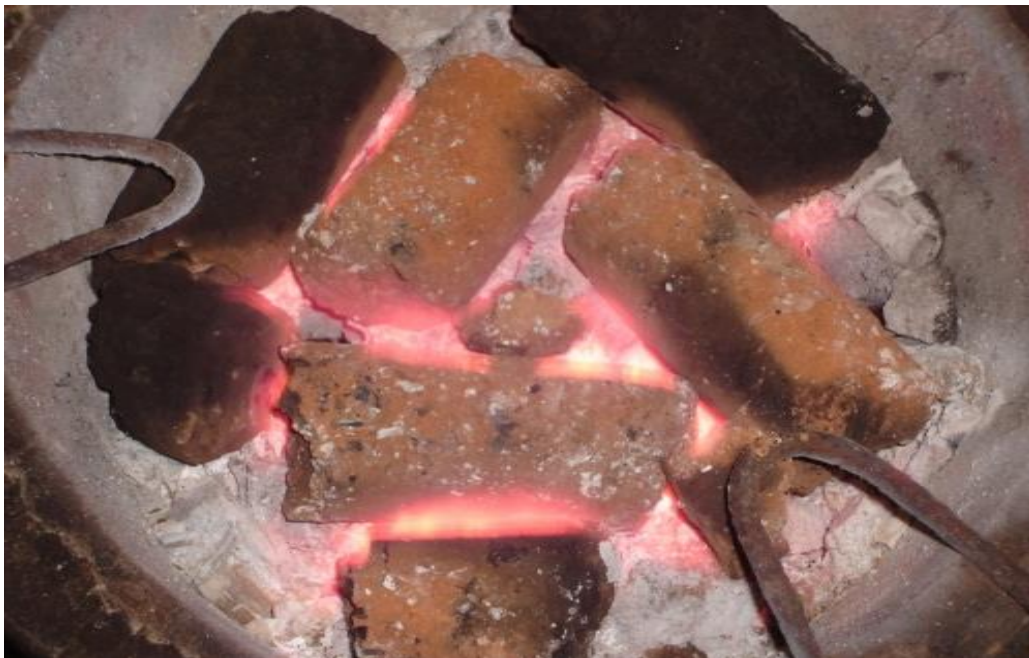
Plate 2.3: Charcoal briquettes in Kenya Ceramic Stove
