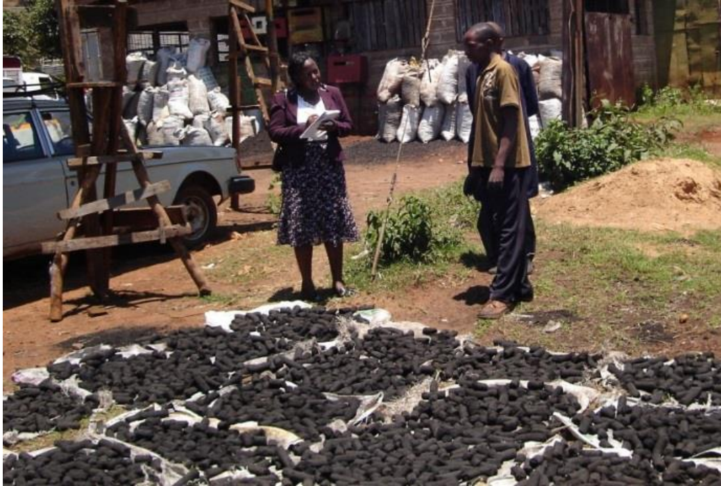
Plate 2.2: Drying Charcoal Dust Briquettes
