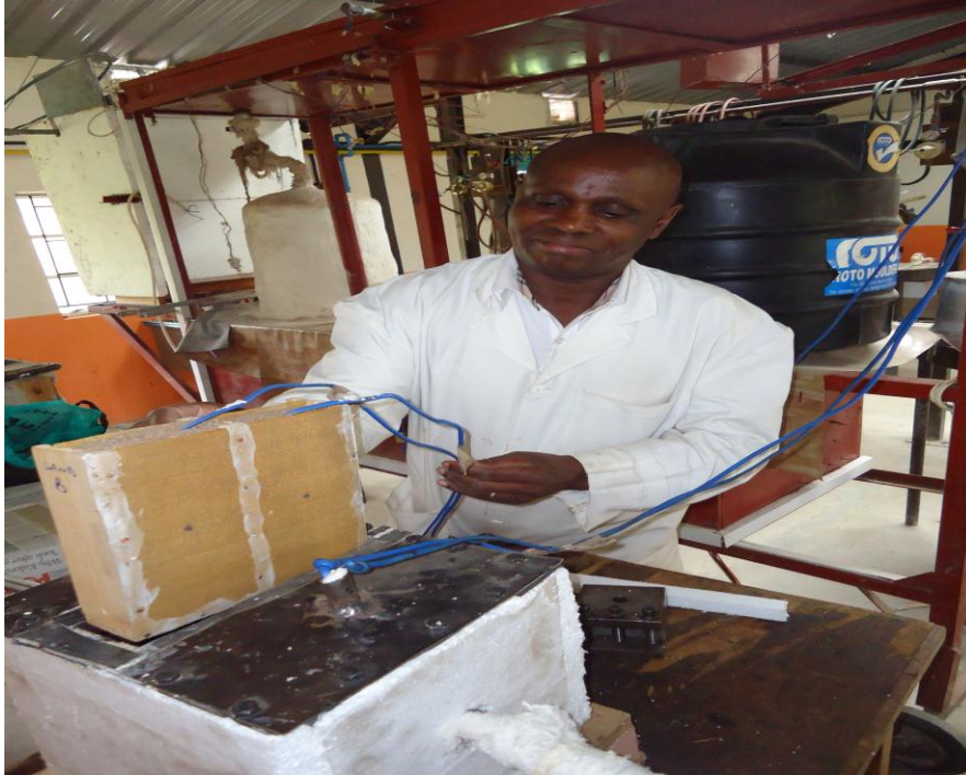
Figure 3.5 Fitting the Sand Container into the Insulated Rectangular Section Tank
