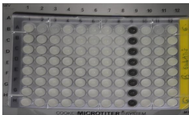
Figure 20: Minimum inhibitory concentration (MIC) assay of 5 pure fungal compounds isolated from KE/16-163 ( Fomitiporia aethiopica ) against B. subtilis test pathogen. (A) Column (C) 1-compound 1 ; C2- compound 2 ; C3- compound 3 ; C4- compound 4 ; C5-compound 5 ; C9, Positive control; C10, Negative control. The letter and number before the fungi strain refers to Column number on the microtiter plate e.g. C4 refers to column 4.
