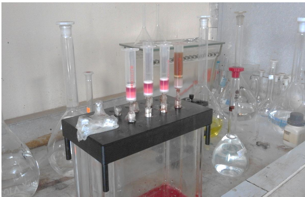
Plate 7: Extraction and purification of anthocyanin using solid phase extraction cartridge
