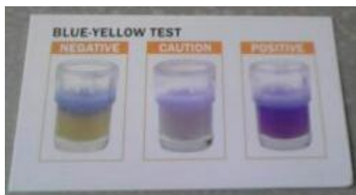
Figure 1: Interpretation chart of Charm II Blue Yellow test
