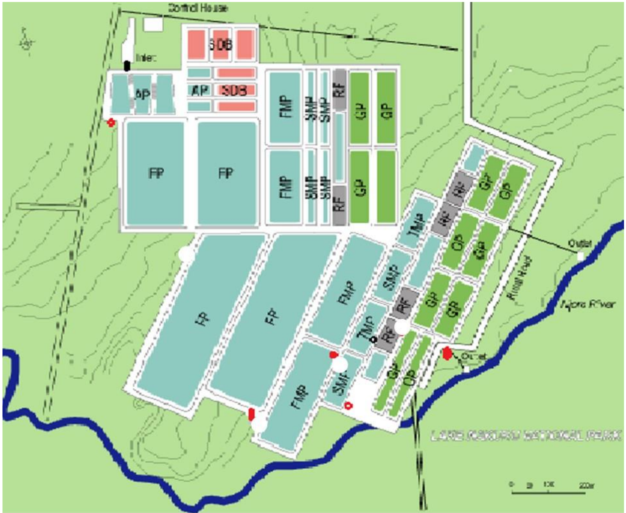
Figure 0.2: Njoro sewage works sketch diagram AP-Anaerobic pond
