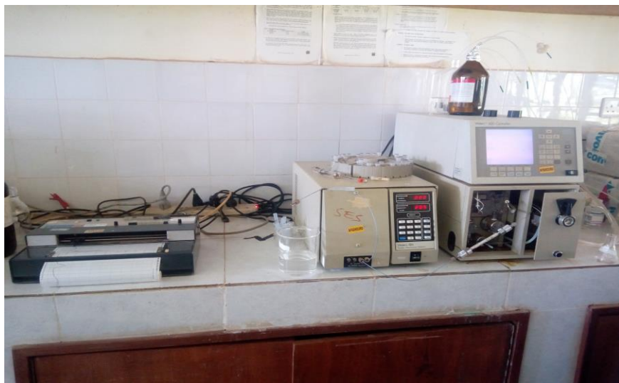
Plate 3.1: Machine setup; plotter, detector and HPLC machine
