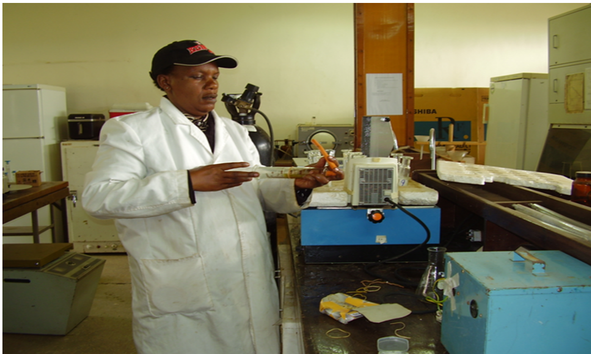
Plate 5: Adjusting calibrated glass syringe during in-vitro gas production
