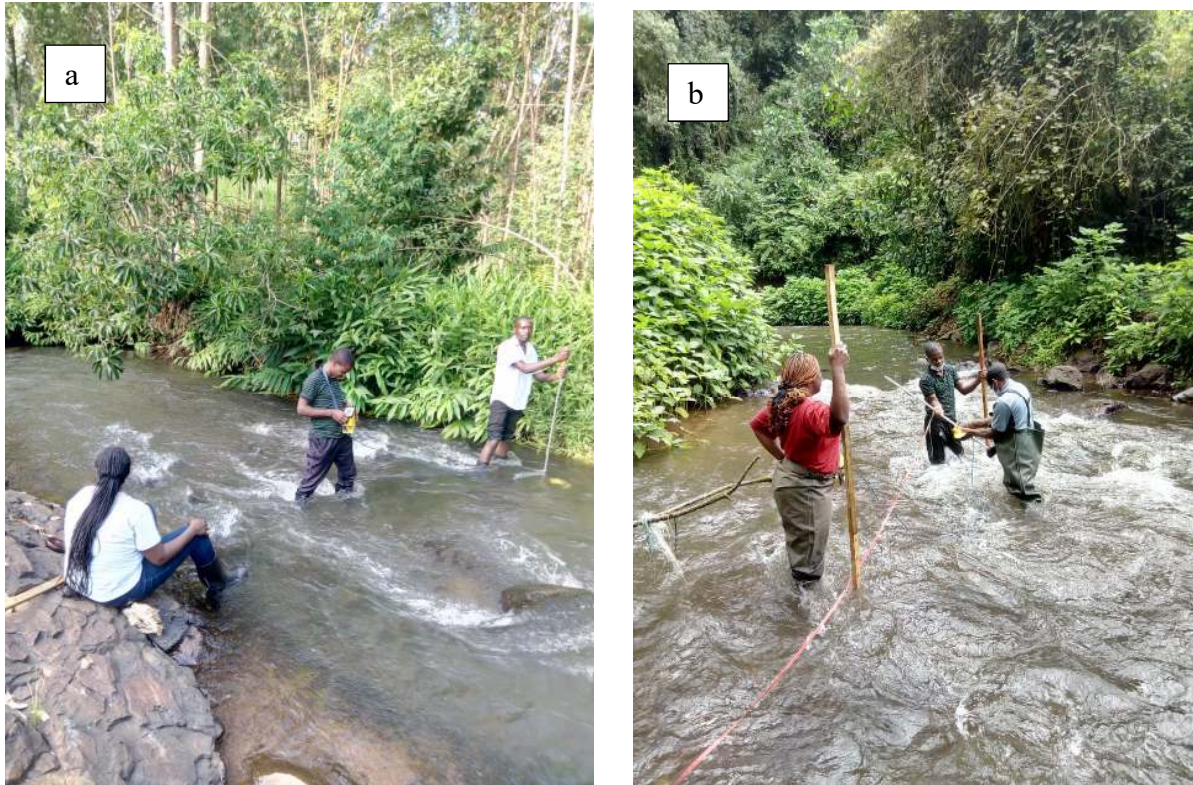
Figure 4(a,b): Measurement of (a) flow velocity and (b) stream width and depth, in the study sites
