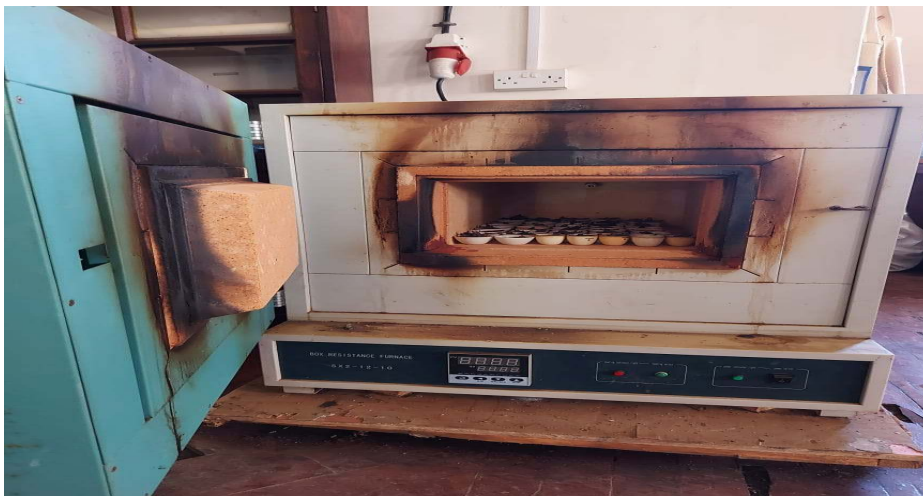
Figure 7: Laboratory determination of ash weight of leaf litter using muffle furnace
