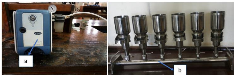
Plate 8 : Photographs showing (a) vacuum pump and (b) multichannel filtration unit
