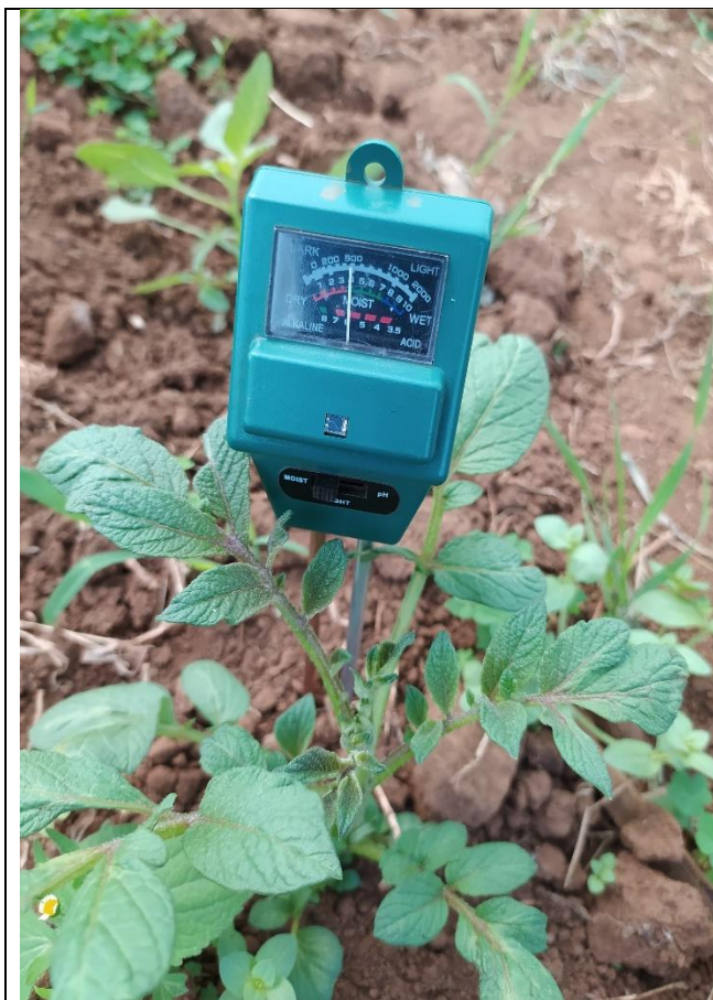
Root zone soil moisture measurement using moisture sensor before irrigation event
