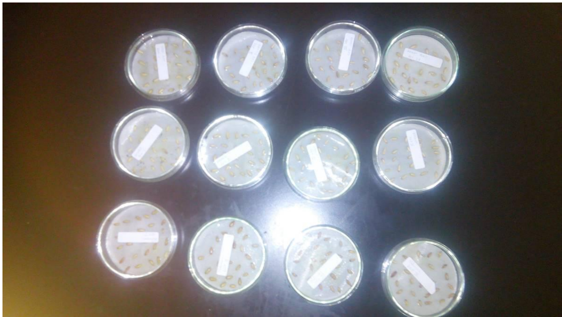
Plate 3.2: Germination seeds test arrangement in groups of 25 on filter paper
