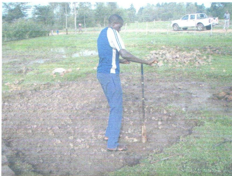
Plate 2: Soil sampling using an auger at K'Onyiero
