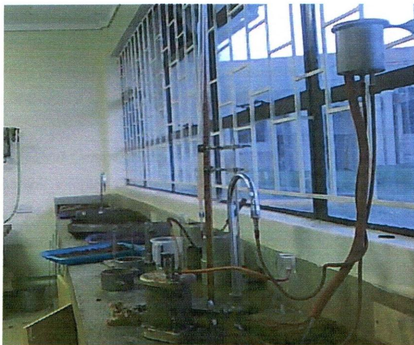
Plate 5: Constant head permeability test arrangement
