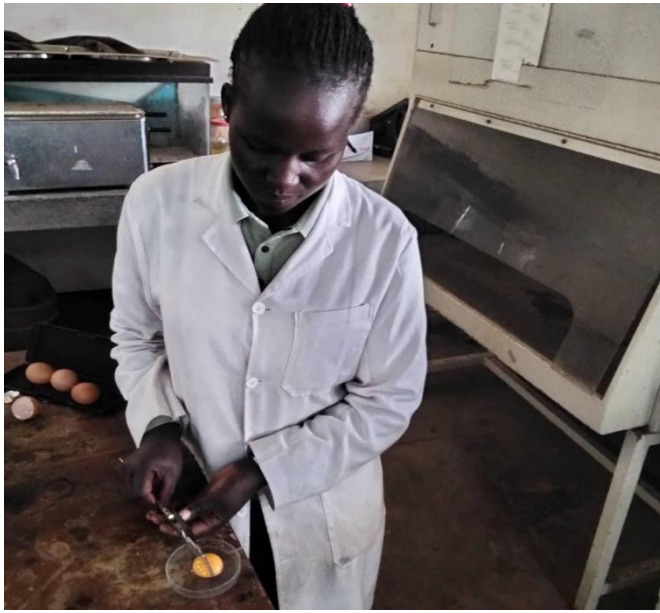
Yolk Index Determination using a Vanier calliper Laboratory and egg quality analysis (Chelangat, 2025)
