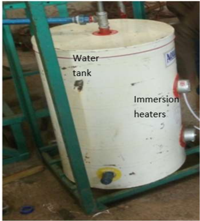
Plate A2.3: Water tank with immersion heaters
