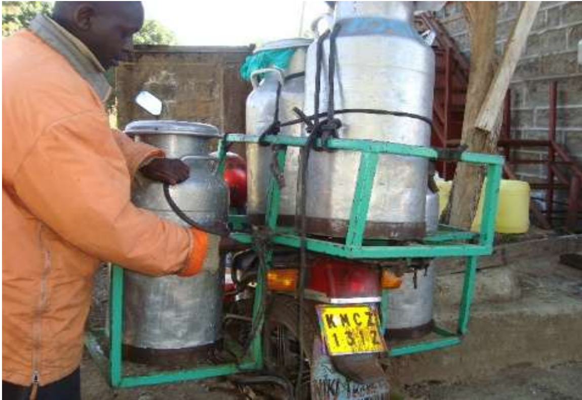
Figure 2: A customized motorbike carrier for Aluminium churns common in the peri-urban dairy value chain
