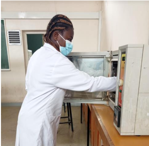
E: Putting samples in an incubator at given temperature
