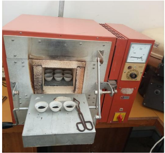
Figure C.8: Combustion analysis of briquettes in a muffle furnace
