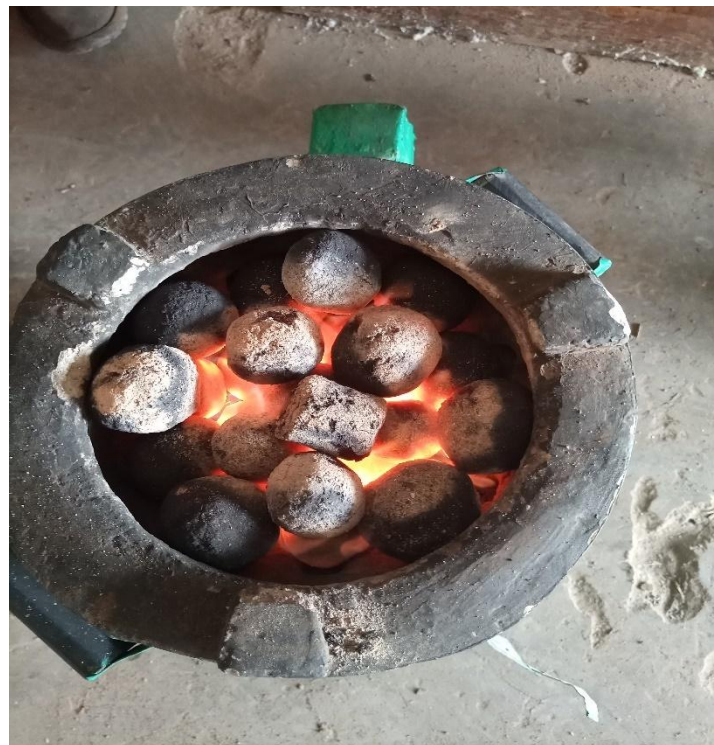
Figure C.10: Burning briquettes in improved jiko
