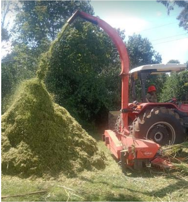
Mounted forage harvester cutting sweet sorghum to small pieces
