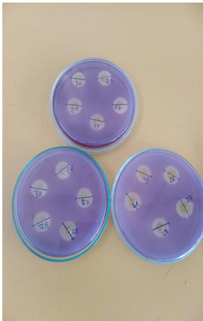
Figure 4. 5: Plate Indicating Clear Zone by Produced Pectinase Enzyme
