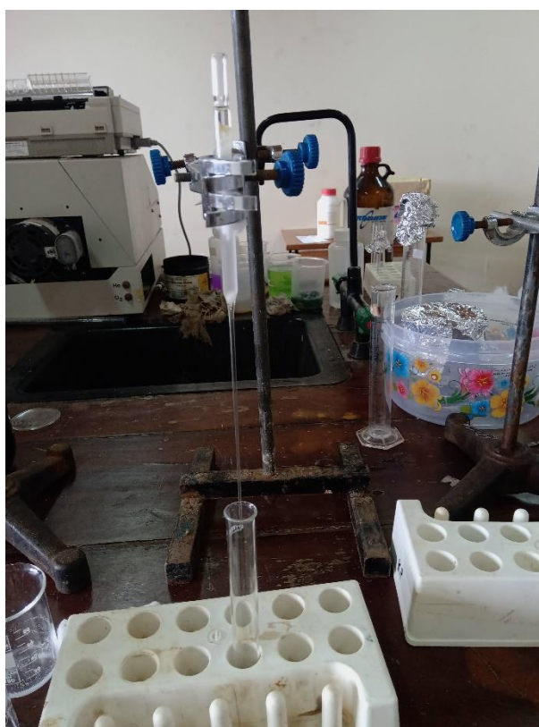
Plate 3: Column packed with pre-activated silica gel
