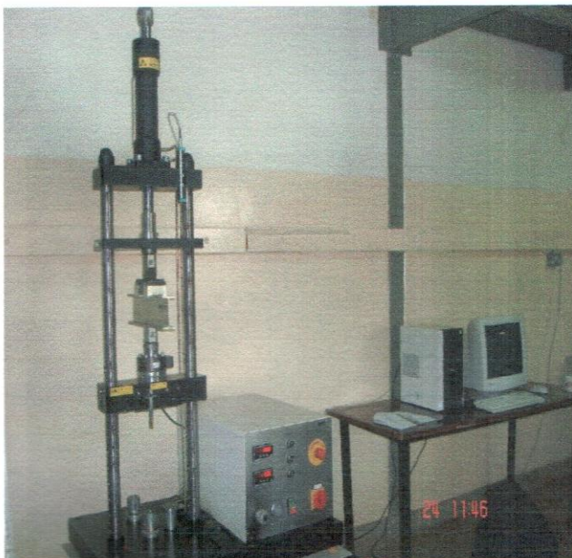
Figure 3.10 The hydraulic Universal Material Tester 50 kN (WP 310) machine
