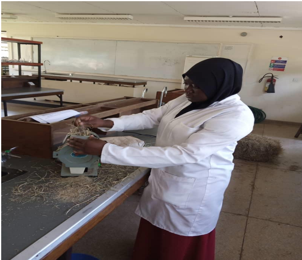
Plate 3.1: Grinding a sample of feed ingredients using a hammer mill
