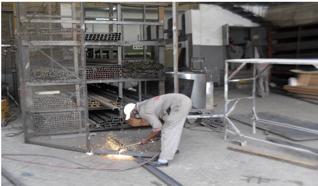
Plate 4: below shows metal cutting by a craftsman in the vehicle body fabrication.
