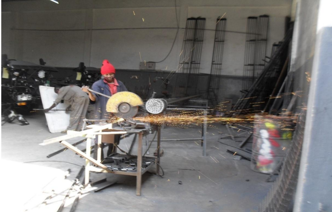
Plate 6: Metal cutting machine in preparation for vehicle body fabrication
