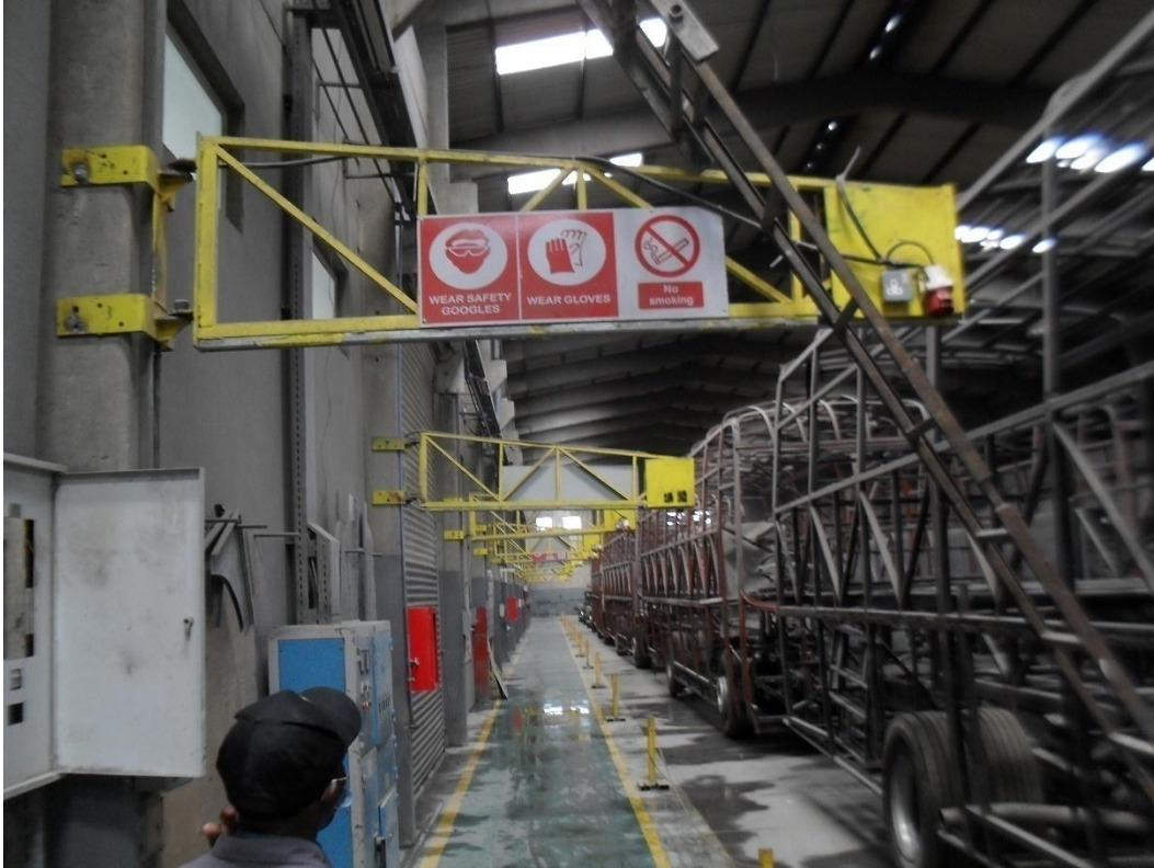
Plate 10: Vehicle bodies fitted with frames awaiting panel fitting
