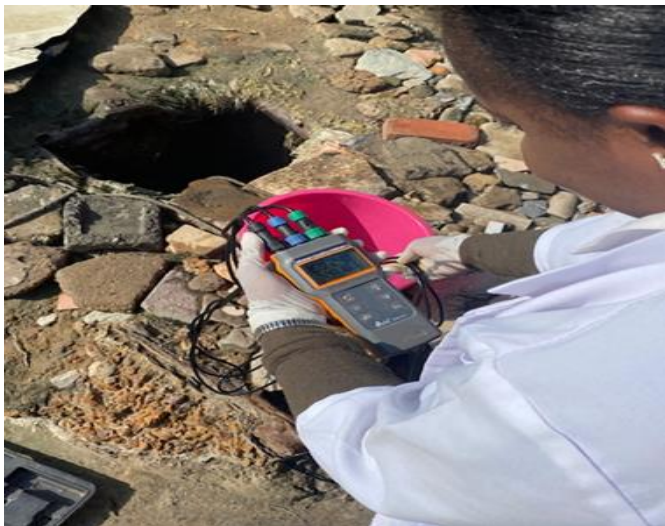
Plate 3.2: On-site measurement of physical parameters using a multi-parameter probe
