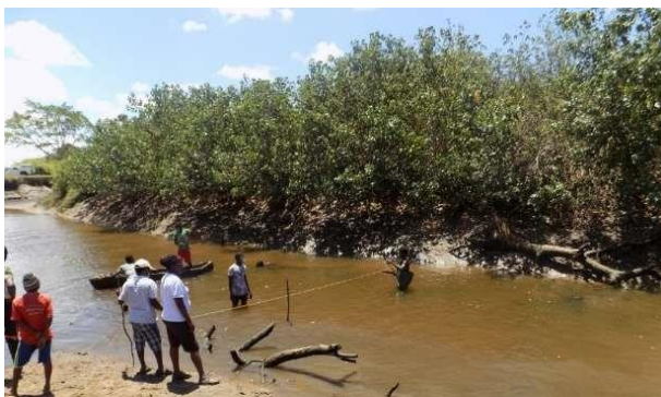
Plate 3: Measuring River channel depth and width at a) Sabaki and b) at Taliani along the Athi-Galana-Sabaki and Ramisi Rivers
