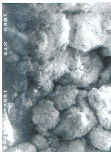
Fig. 6: Scanning electron micrographs of the crusts and the soil underneath (A), and of the bulk soil at 5 mm depth that was not affected by rainfall (B), for the Tunyai, Neve Ya'ar and Molo soils. The micrograph in (B) for Neve Ya'ar soil shows the “washed-in” zone.
