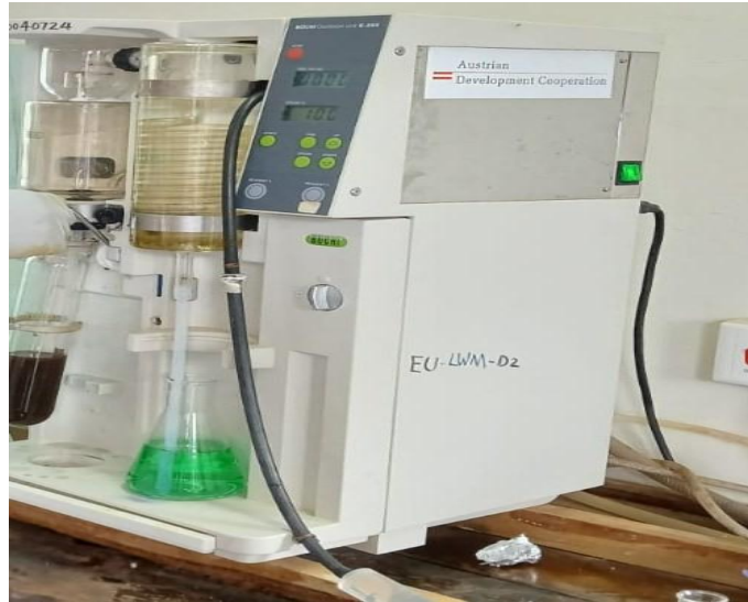
Plate 3.4: Kjeldahl distillation unit used for Total Nitrogen determination in macrophytes
