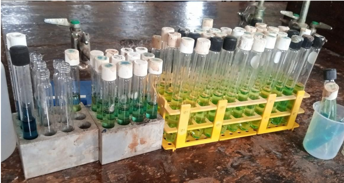
Plate 3.3: COD samples analysis equipment set up at the LWM laboratory at Egerton University
