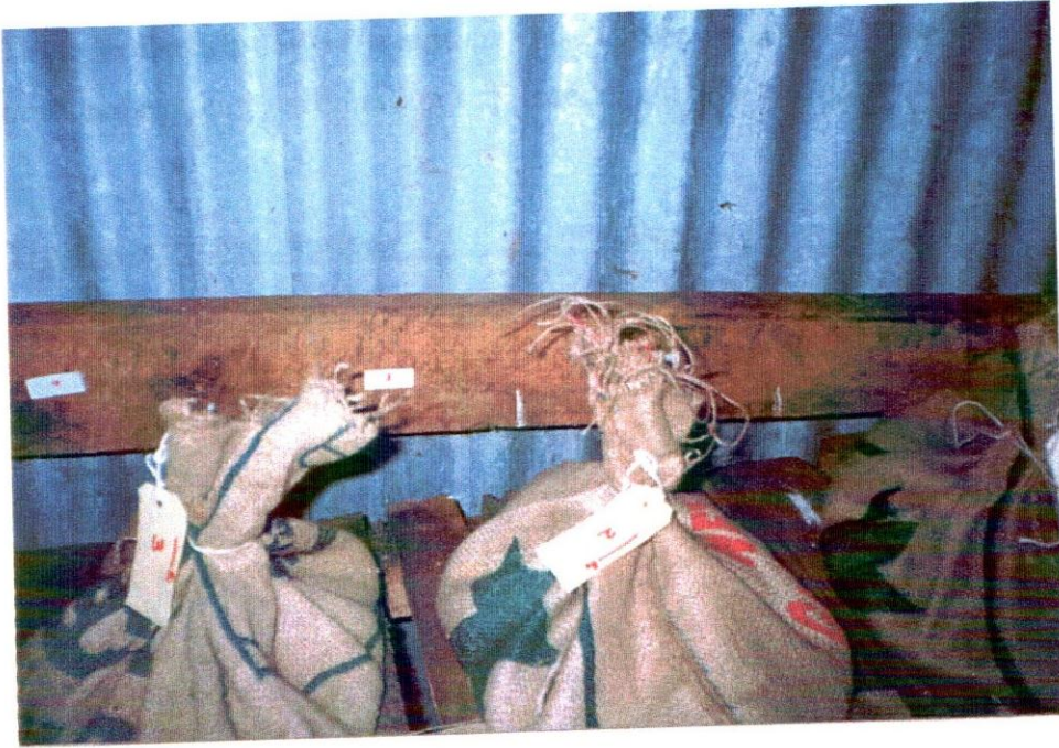
Plate 3: Grain quality evaluation experiment: 5-kg grain samples in jute bags on 1-m high wooden platform
