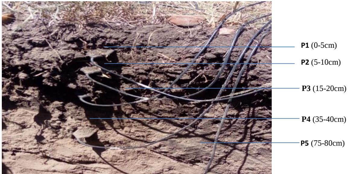
Figure 3.6: Soil moisture and temperature capacitance (5TM-ECH 2 O) probes
