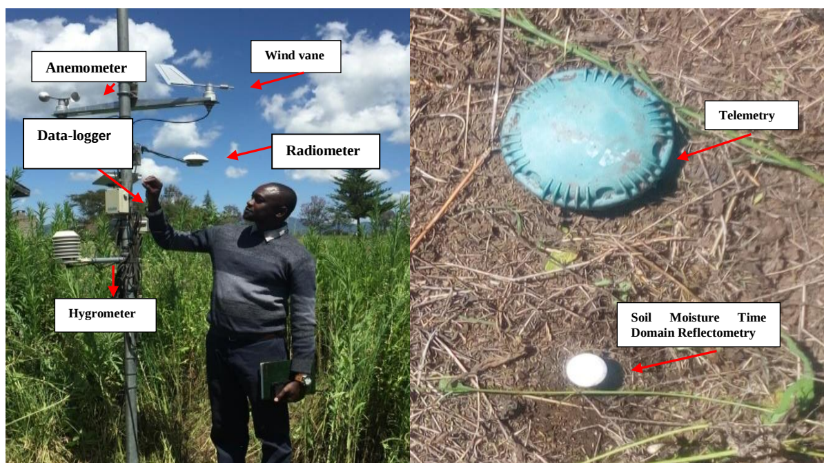
Figure 4.30: Automatic Weather Station at Kijabe Farm Naivasha Cropland
