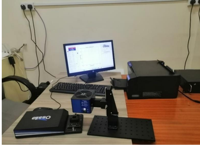
Figure 3.12: A solar simulator used to test fabricated cell performance
