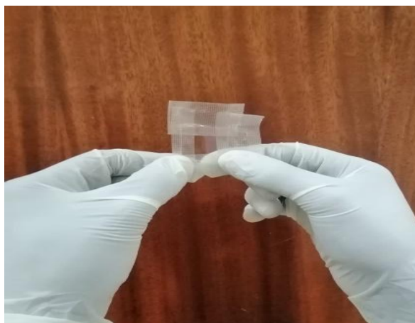
Figure 3.4: Demarcating FTO glass for TiO 2 deposition.
