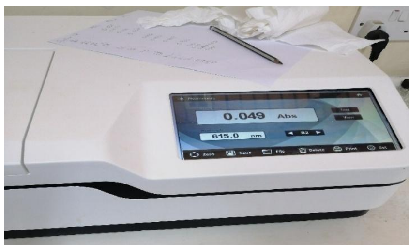
Figure 3.8: UV-Vis spectrophotometer setup used for absorbance measurement.
