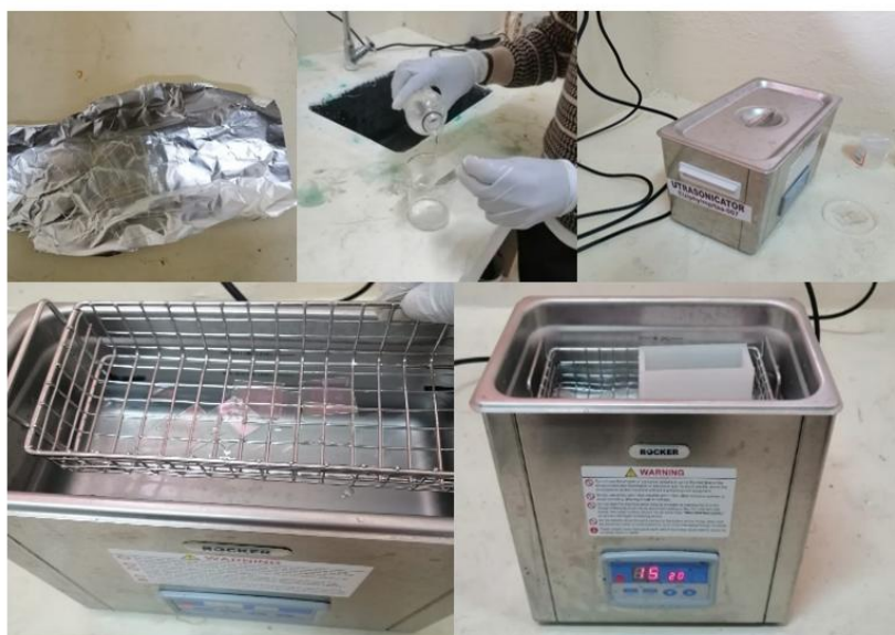
Figure 3.2: FTO Glass substrates cleaning process
