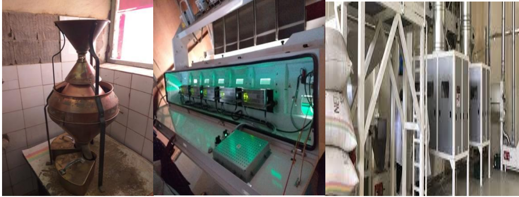
Figure 3. 4: Sesame value addition (a) laboratory-based homogenizer to screen and grade sesame based on impurity level, (b) Industrial based sesame sorting based on colour and (c) industrial based sesame de-hulling
