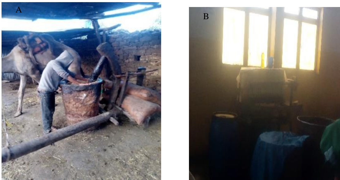
Figure 3. 1: Crude Sesame Extraction in Tigray, Ethiopia A) Camel driven and B) Small scale cold mechanical pressing method of crude sesame oil extraction
