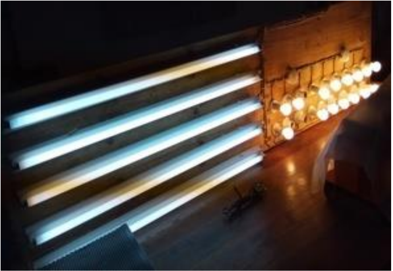
Plate A-5: 240V 100W bulbs and 1.2M × 36W fluorescent fittings connected in parallel for data collection
