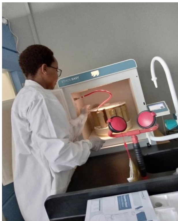
Plate 2: Samples placed in an advanced microwave digestion system (ETHOS EASY, Milestone)
