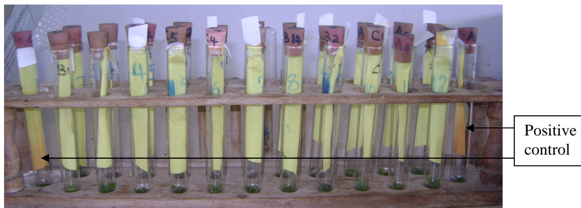
Plate 4.1: Analysis of cyanogenic glycosides for L. purpureus seed samples using the picrate method: cassava positive controls are shown at each end of the test tube rack
