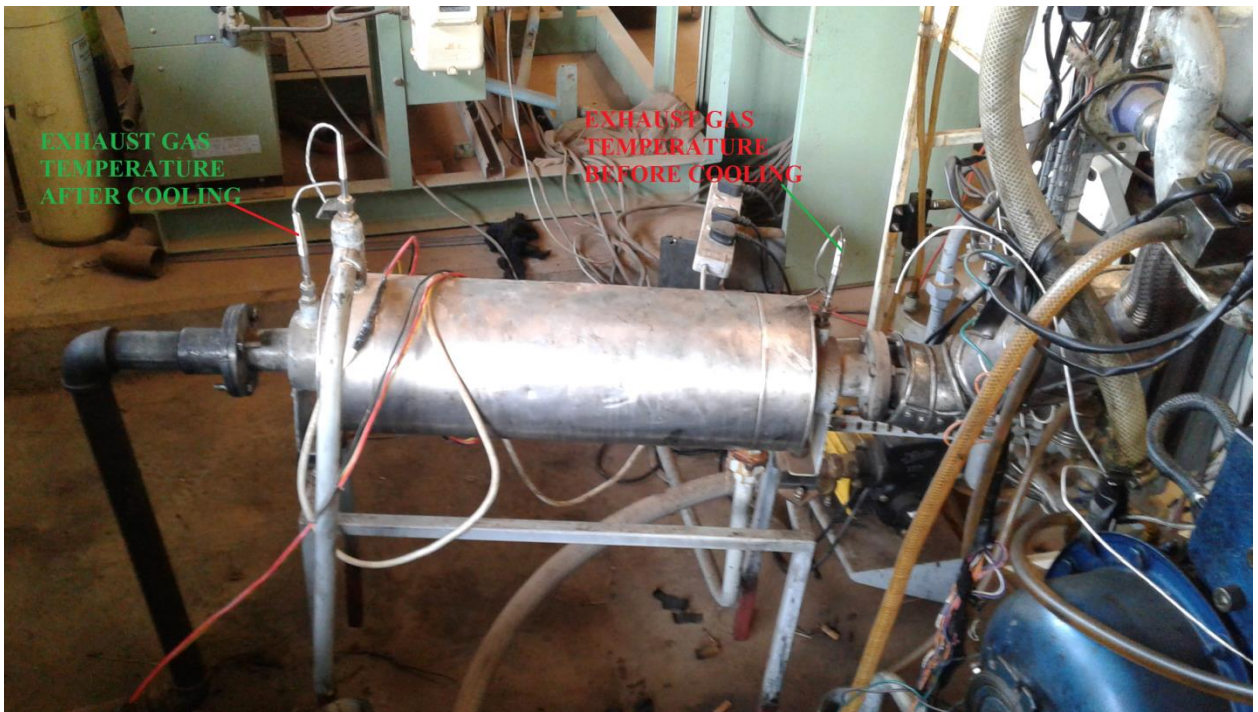
Figure B 3: Calorimeter for energy recovery
