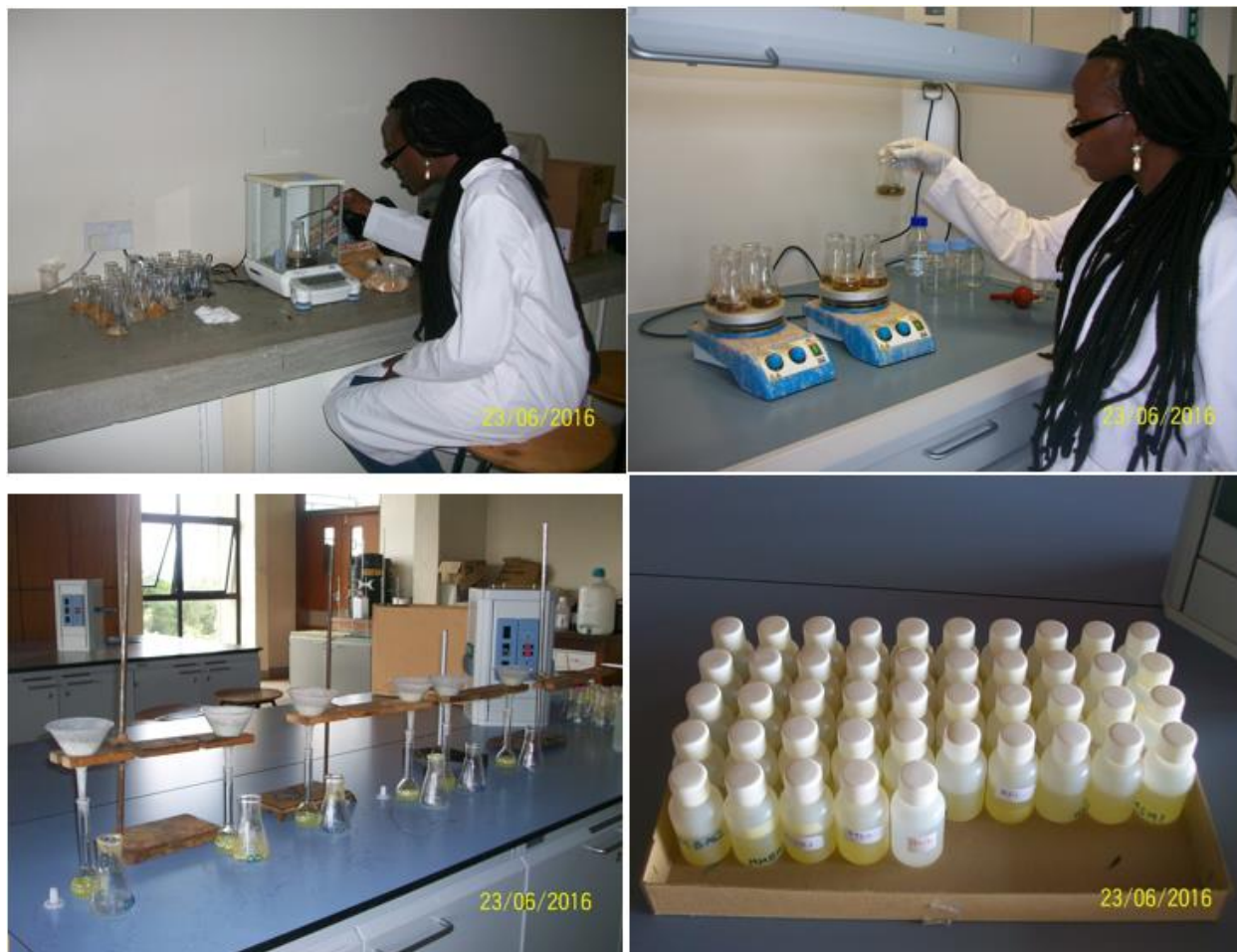
Plate 1: Digestion process of the samples of the widely consumed fish species
