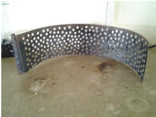
PLATE D2: Materials sieve for particle briquette segregation
