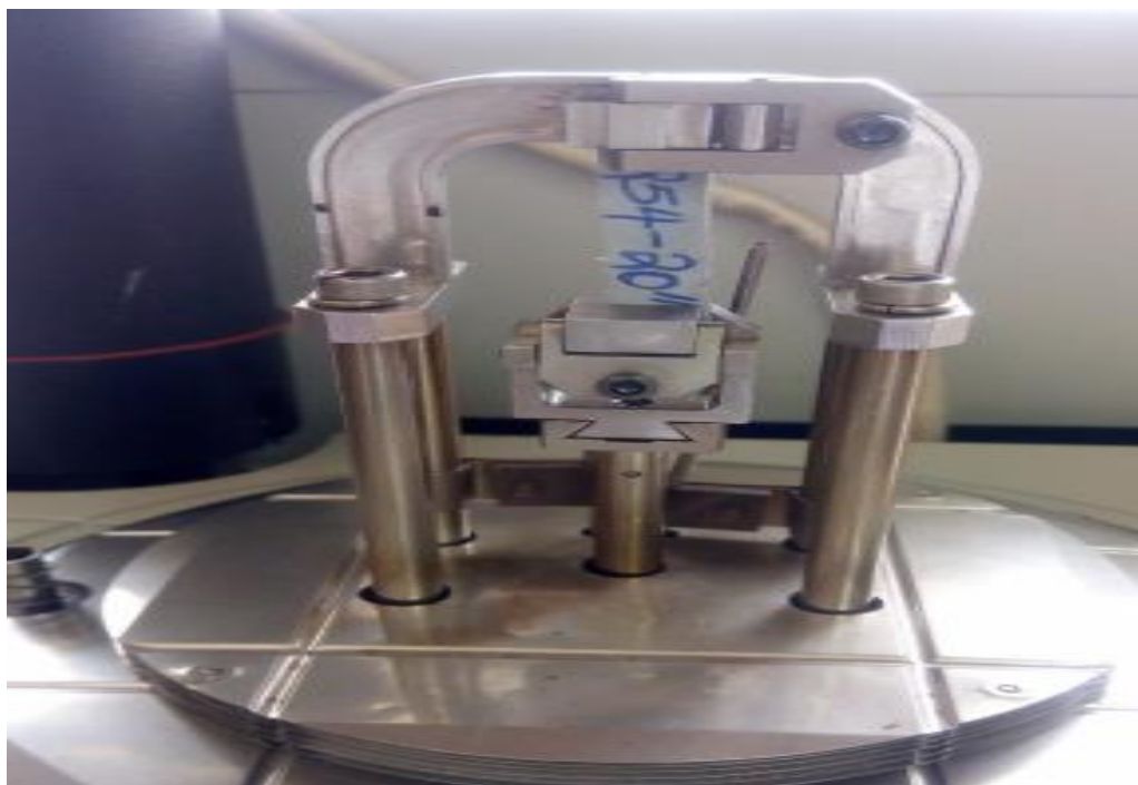
Plate 3.4: Picture showing Film tension clamp of a DMA 2980
