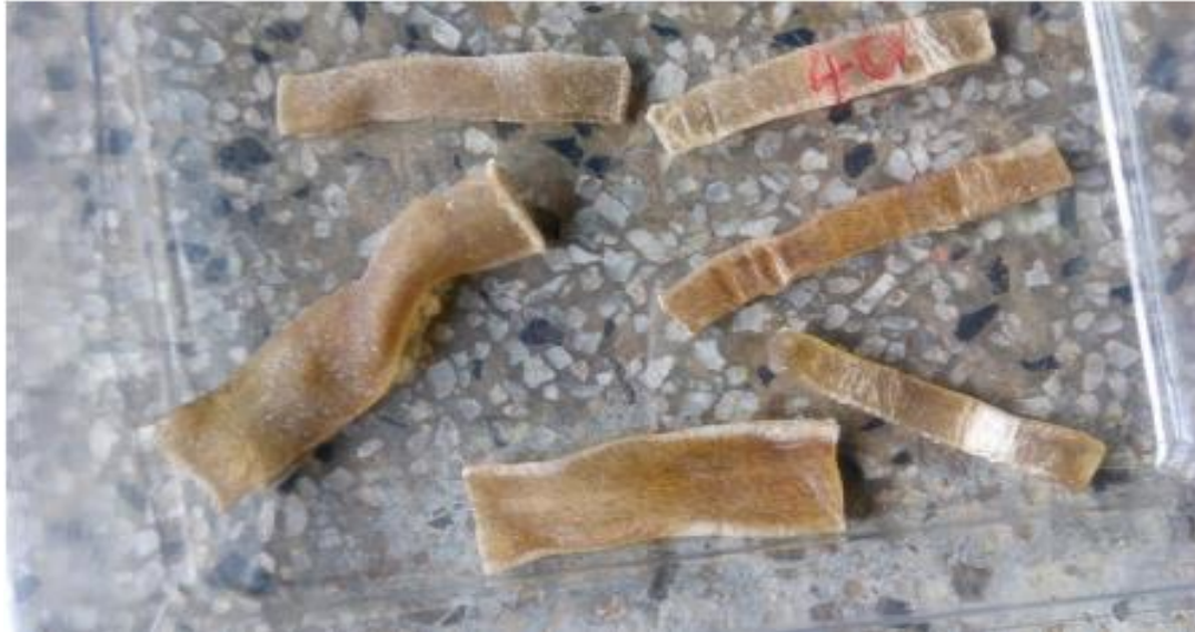
Plate 3.2: Picture showing pickled hide sample for Film tension clamp of DMA 2980
