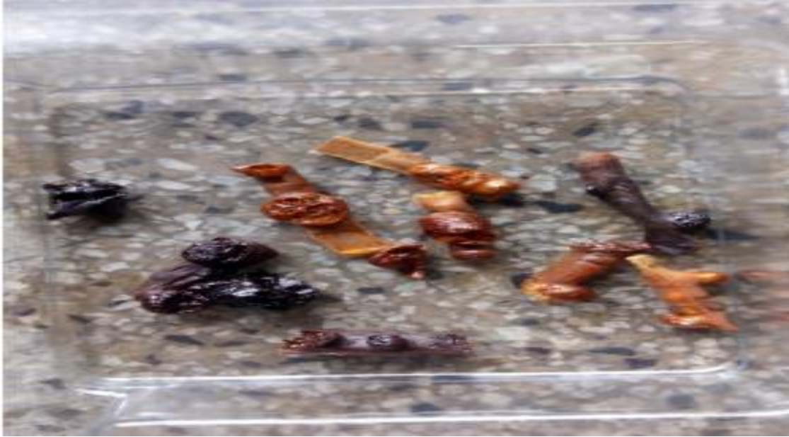
Plate 4.1: Picture showing decomposed pickled sample after DMA 2980 experiment
