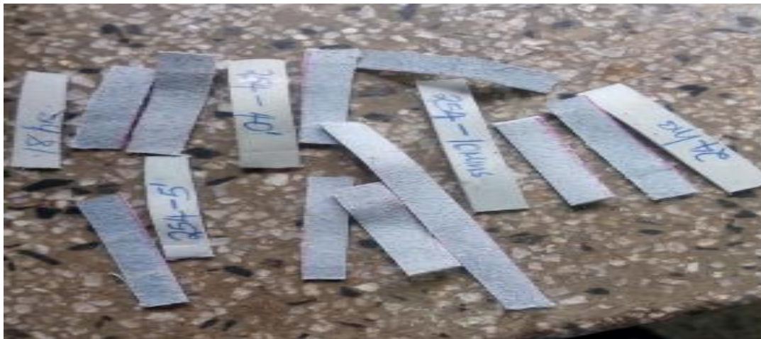
Plate 3.3: Picture showing pickled hide sample for Film tension clamp of DMA 2980
