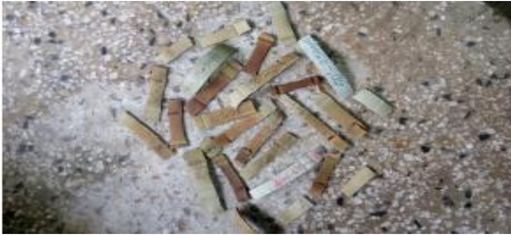
Plate 4.2: Picture showing tanned hide sample after DMA 2980 experiment
