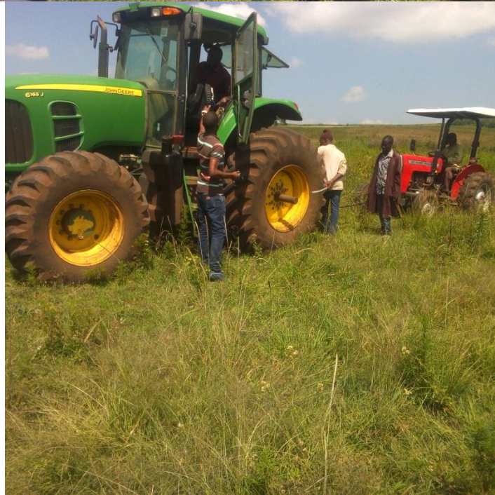
Figure B. 2: Setup of the two tractors and dynamometer system
