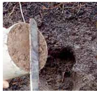
Plate 3. 2: Removing excess soil from the ends of core ring
