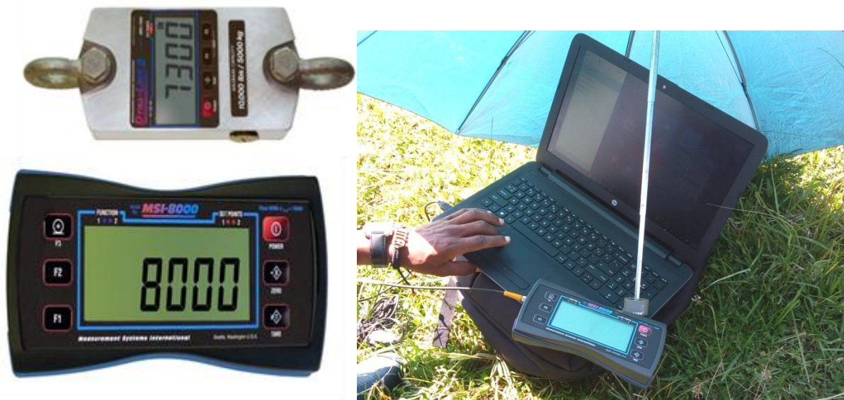
Plate 3.5: Dyna-Link 2 tension dynamometer set-up
