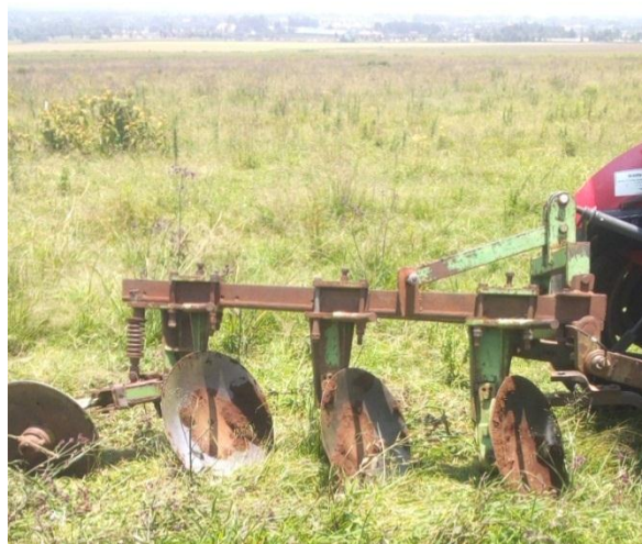
Figure B.4: A 3- Bottom disc plough attached to the three point hitch system of the tractor
