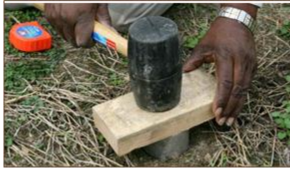
Plate 3. 1: Driving the core ring to required depth
