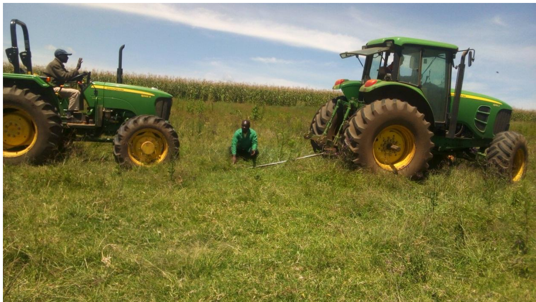
Plate 3. 4: Field set-up comprising of two tractors and load cell
