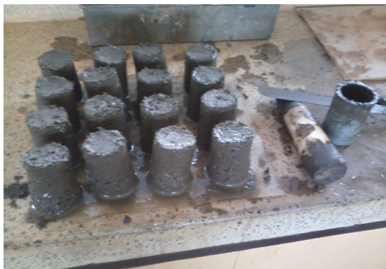
c) Moulding the blocks
