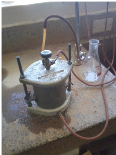
k) Permeability test set up
