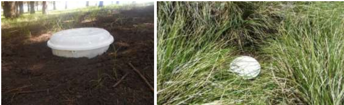
Plate 5: Plastic chamber inserted into the forest floor
